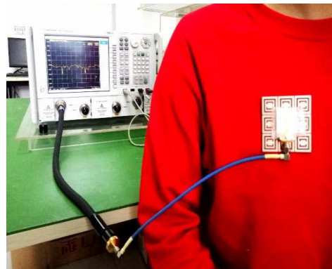
Figure 18. Measured photograph of the fabricated antenna placed on the human body.
