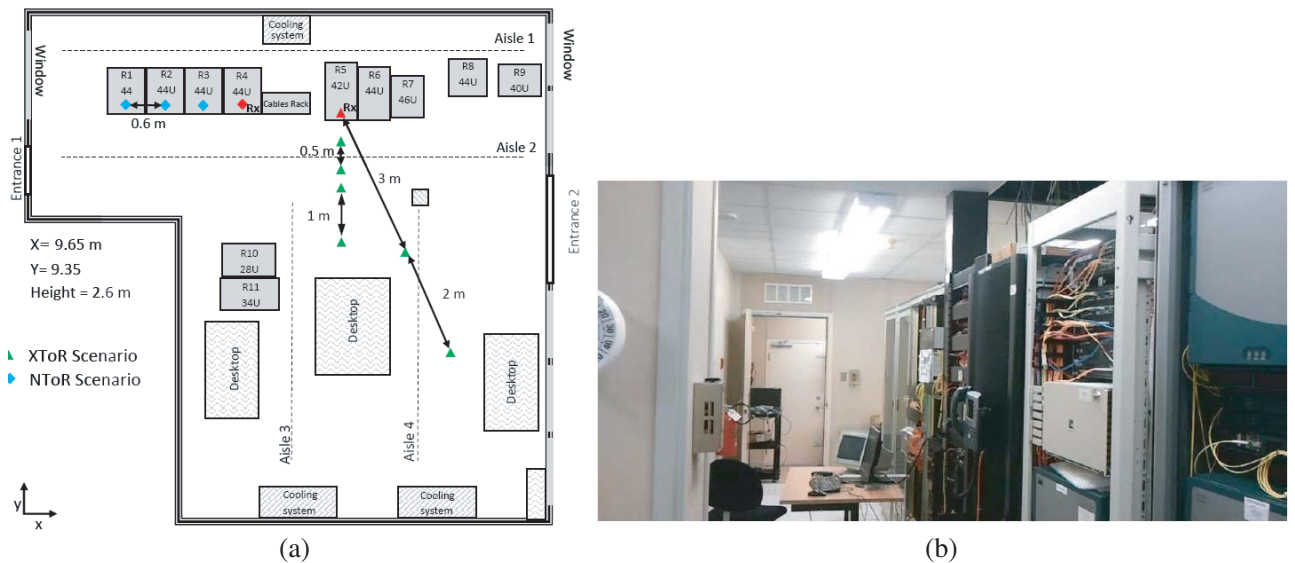
Figure 1. Campus server room layout: (a) Campus data center environment floor plan (not in scale) with measurement scenarios, and (b) photograph of a rack-row.
