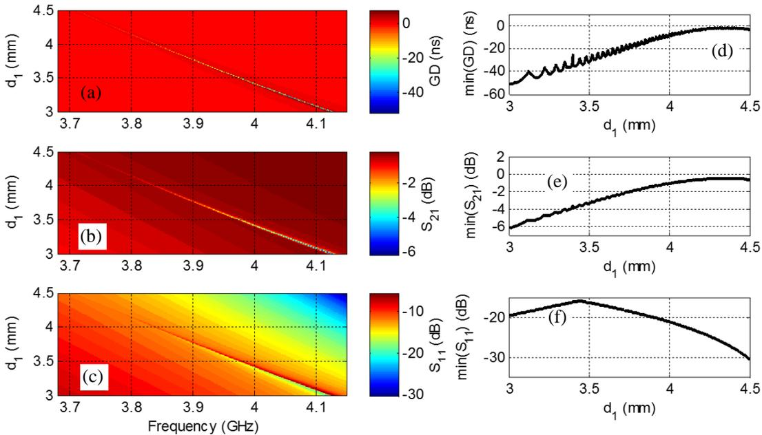
**Figure 9.** Cartographies of (a) GD, (b)  $S_{21}$  and (c)  $S_{11}$  vs  $(f, d_1)$ , and (d)  $\min(\text{GD})$ , (e)  $\min(S_{21})$  and (f)  $\min(S_{11})$  vs  $d_1$ .
