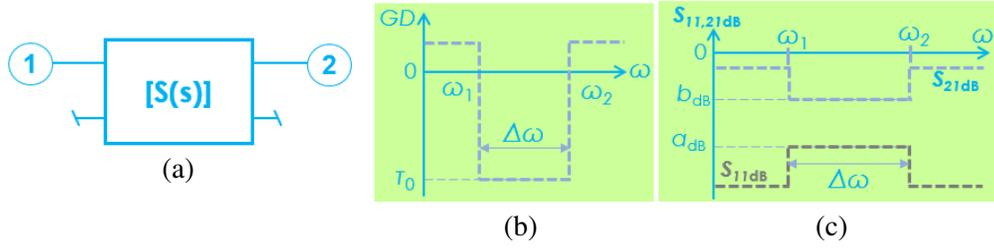
**Figure 1.** (a) Two-port black box microwave system. BP NGD function ideal specifications: (b) GD, and (c)  $S$ -parameters,  $S_{11}$  and  $S_{21}$ .
