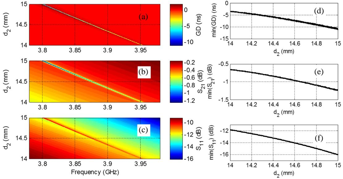
**Figure 10.** Cartographies of (a) GD, (b)  $S_{21}$  and (c)  $S_{11}$  vs  $(f, d_2)$ , and (d)  $\min(\text{GD})$ , (e)  $\min(S_{21})$ , and (f)  $\min(S_{11})$ .
