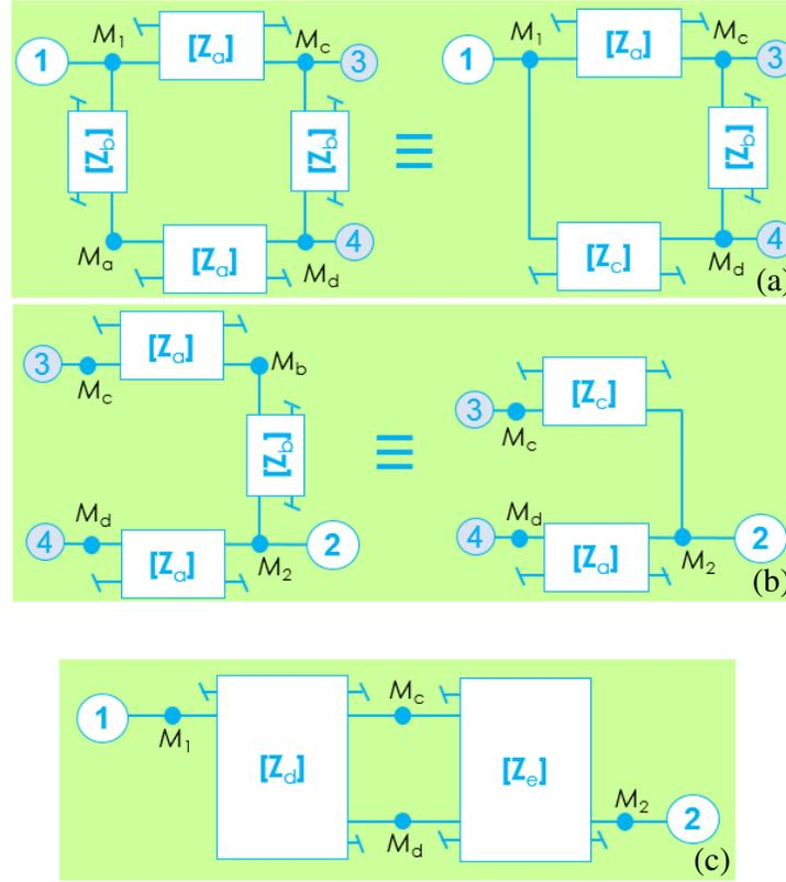
**Figure 4.** Reduced topology of (a) left and (b) right parts of the ladder network equivalent diagrams, and (c) 3-port  $S$ -matrix block diagram-based ladder network equivalent schematic.
