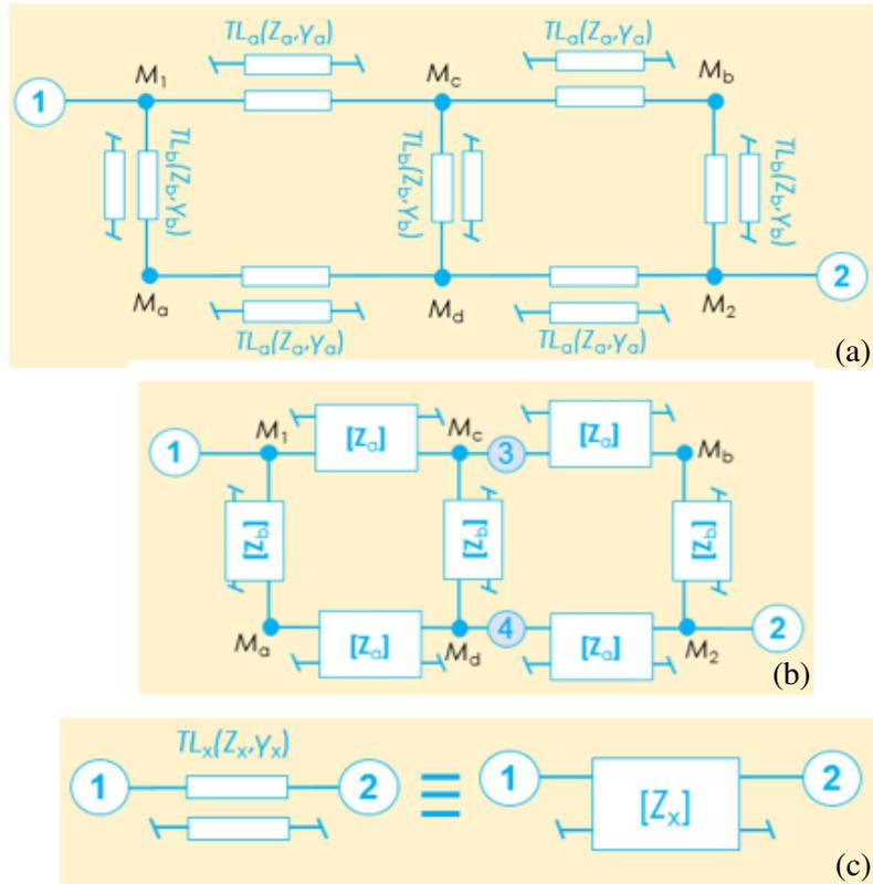
**Figure 3.** (a) TL based topology of ladder network under study, (b) two-port TL  $Z$ -matrix blocks-based equivalent diagram, and (c) TL and its two-port  $Z$ -matrix equivalent model.
