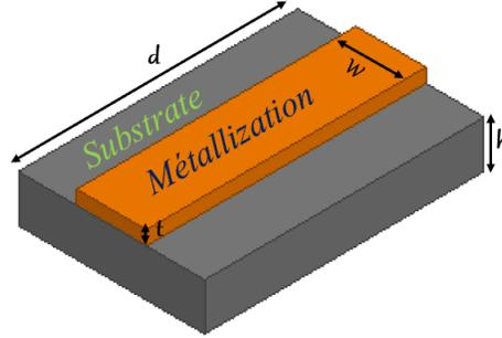
**Figure 2.** Typical microstrip line and geometrical parameters.
