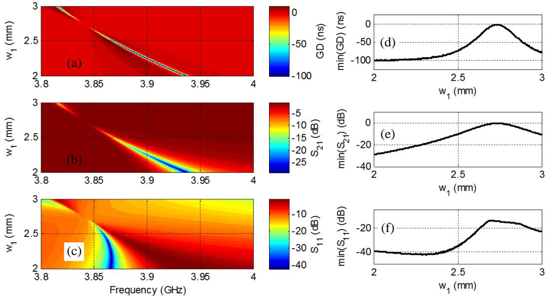
**Figure 7.** Mappings of (a) GD, (b)  $S_{21}$  and (c)  $S_{11}$  vs  $(f, w_1)$ , and (d)  $\min(\text{GD})$ , (e)  $\min(S_{21})$  and (f)  $\min(S_{11})$  vs  $w_1$ .
