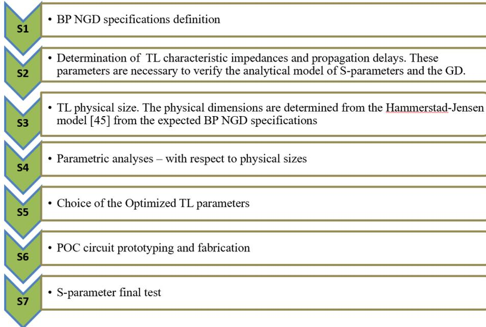
**Figure 5.** Steps diagram design of the Ladder-shaped topology.
