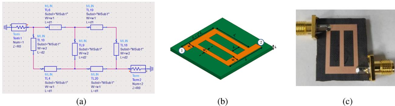
**Figure 6.** Ladder shape circuit prototype: (a) ADS® schematic, (b) 3-D design and (c) photograph.
