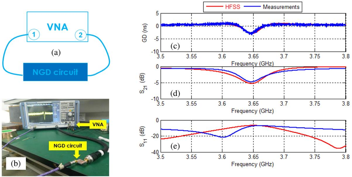
**Figure 11.** NGD circuit experimental setup: (a) diagram and (b) photograph. Comparison between calculated, simulated and measurements: (c) GD, (d)  $S_{21}$  and (e)  $S_{11}$ .
