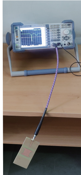
Figure 5. Experimental setup. Setup for |S_{11}| plot, VSWR and Z measurement.
