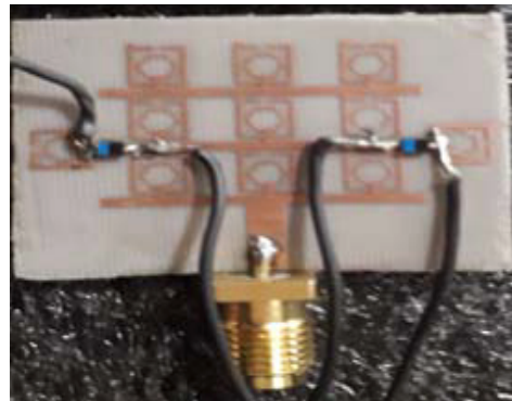
Figure 6. Fabricated reconfigurable antenna.
