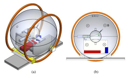
**Figure 1.** Schematic sketch of the experiment ((a) overall, (b) sectional view with indication of electron flight path).
