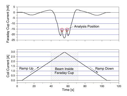
Figure 3. Faraday cup current as a function of the Helmholtz coil current.
