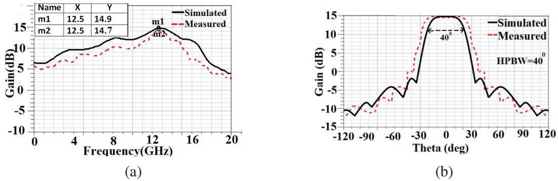
**Figure 6.** (a) Frequency-gain plot. (b) Plot of sector shaped gain pattern.
