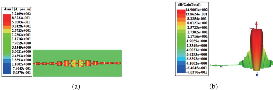
**Figure 5.** (a) Surface current distribution of simulated array. (b) 3D Gain of simulated array.
