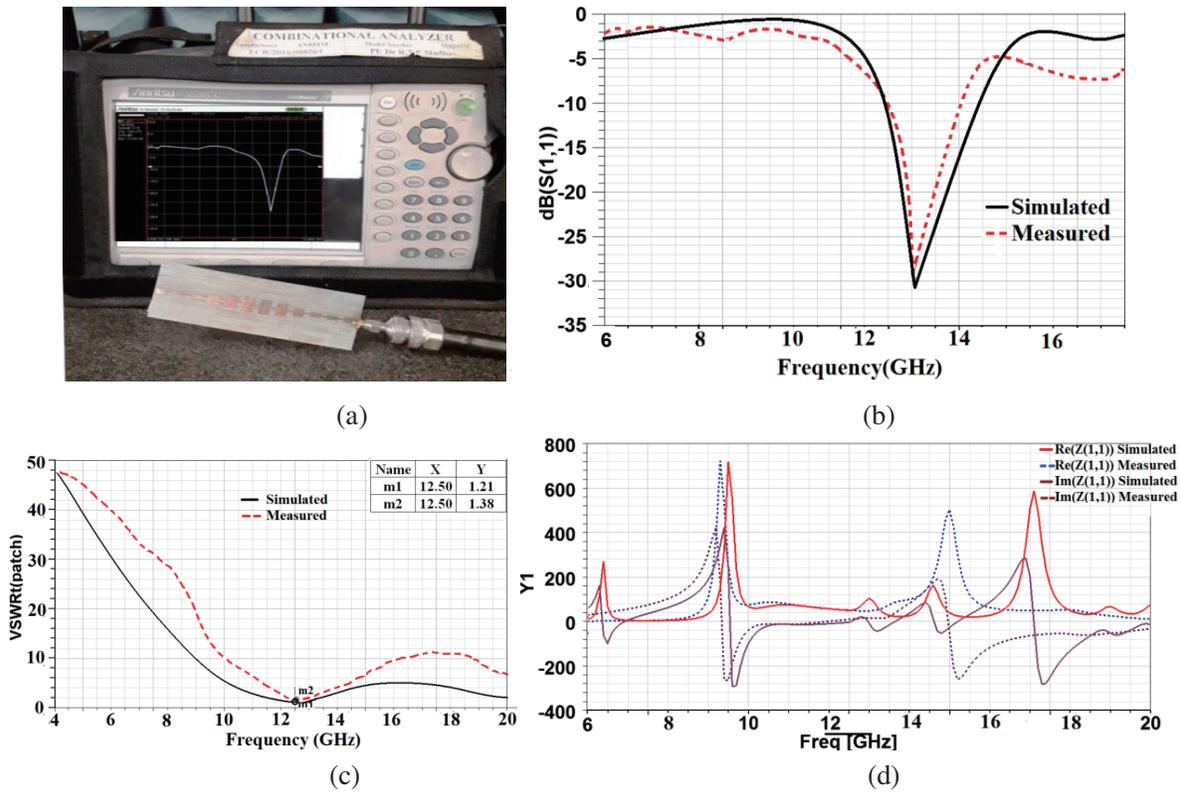
**Figure 4.** (a) Return loss simulation measurement. (b) Return loss simulation and measurement plot. (c) VSWR measurement. (d) Input impedance simulated and measured.
