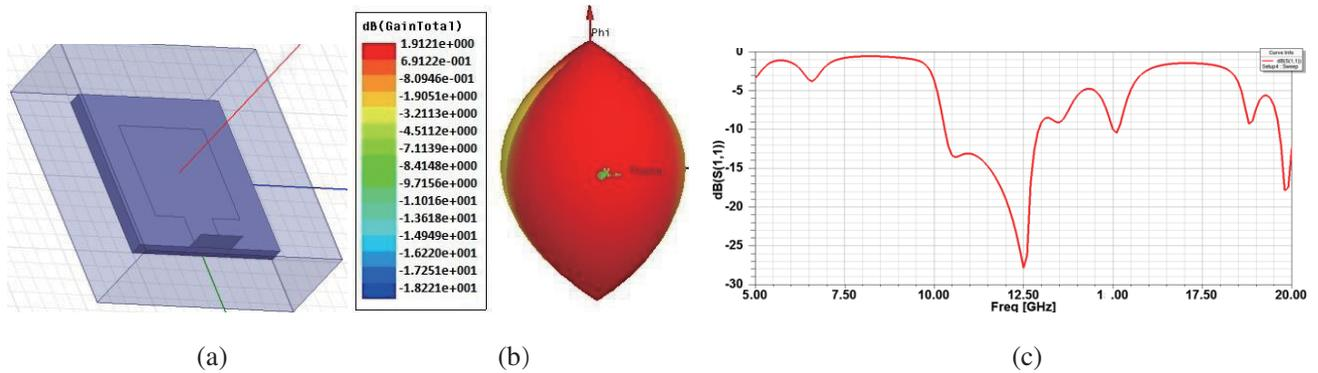
**Figure 2.** (a) Single antenna 3D view. (b) Radiation pattern of single antenna. (c) Return loss plot of antenna.
