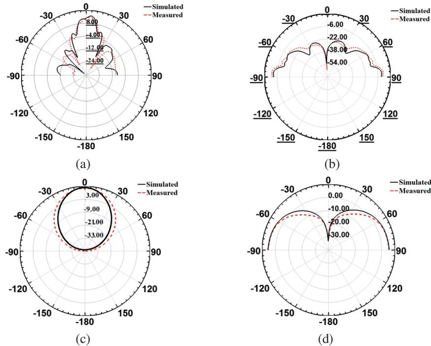
**Figure 7.** (a) Co-polarization of  $E$ -plane. (b) Cross polarization of  $E$ -plane. (c) Co-polarization of  $H$ -plane. (d) Cross polarization of  $H$ -plane.
