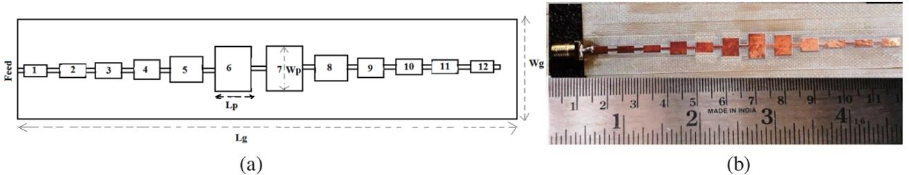
**Figure 3.** Proposed antenna array. (a) Design simulation. (b) Fabricated structure.
