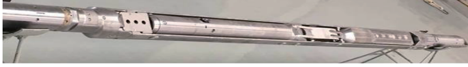
Figure 2. Physical diagram of SHAD-2000 high-frequency dielectric logging tool.
