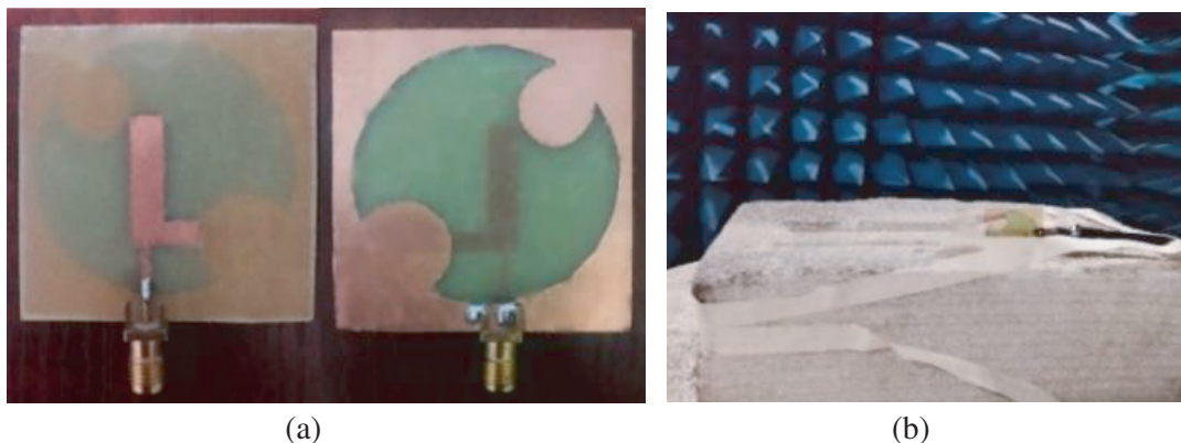
Figure 6. Proposed CP antenna: (a) Prototype; (b) The far field measurement.
