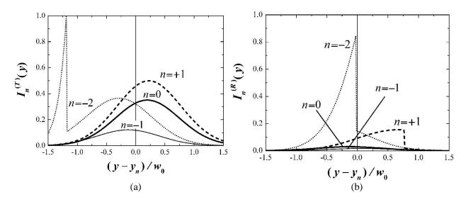
Figure 15. Transverse intensity structure of (a) transmitted  $I_n^{(T)}(y)$  and (b) reflected  $I_n^{(R)}(y)$  beams of various diffraction orders in the planes x = h + H + L and x = -L, respectively, computed relative to the middle of every beam  $y_n$  at the diffraction of the TE polarized beam with the parameter of tangential propagation  $\beta_0 = 0.320$  by a rectangular relief grating located on a substrate with the thickness  $10^3\lambda$ .
