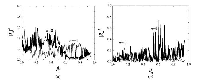
Figure 12. Intensities of the TE polarized (a) two transmitted  $|T_n|^2$  and (b) two reflected  $|R_n|^2$  radiation diffraction orders on the output of a rectangular relief grating located on a substrate of the thickness  $10^3\lambda$ , in dependence of the parameter  $\beta_0$  of incident plane wave tangential propagation.
