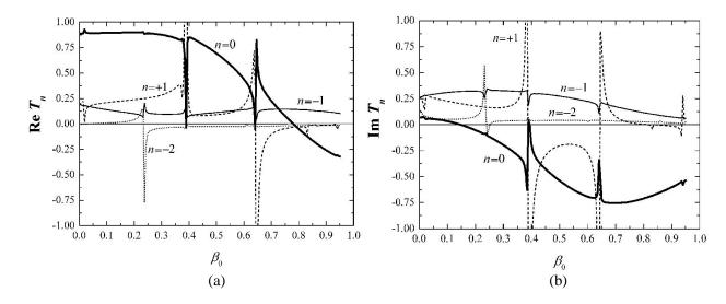
Figure 7. (a) Real and (b) imaginary parts of the complex amplitude transmission coefficient  $T_n$  of a planar sinusoidal grating for 4 diffraction orders as functions of the parameter  $\beta_0$  of tangential propagation of the TE polarized plane incident wave.
