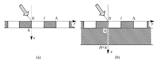
**Figure 1.** Simple binary relief grating (a) without and (b) with a substrate. h is the thickness of a grating,  $\Lambda$  is its spatial period, l is the length of an air groove between two neighbour rulings, H is the thickness of a substrate.
