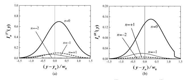
Figure 14. Transverse intensity structure of (a) transmitted  $I_n^{(T)}(y)$  and (b) reflected  $I_n^{(R)}(y)$  beams of various diffraction orders in the planes x = h + H + L and x = -L, respectively, computed relative to the middle of every beam  $y_n$  at the diffraction of the TE polarized beam with the parameter of tangential propagation  $\beta_0 = 0.320$  by a planar sinusoidal grating located on a substrate with the thickness  $10^3\lambda$ .
