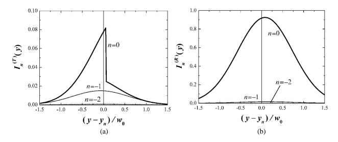
Figure 9. Transverse intensity structure of (a) transmitted  $I_n^{(T)}(y)$  and (b) reflected  $I_n^{(R)}(y)$  beams of various diffraction orders in the planes x = h + L and x = -L, respectively, computed relative to the middle of every beam  $y_n$  at the diffraction of the TE polarized beam with the parameter of tangential propagation  $\beta_0 = 0.64275$  by a planar sinusoidal grating without a substrate.
