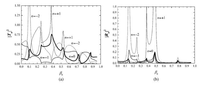
Figure 5. Intensities of the TE polarized (a) 4 transmitted  $|T_n|^2$  and (b) 4 reflected  $|R_n|^2$  radiation diffraction orders on the output of a rectangular relief grating without a substrate as functions of the parameter  $\beta_0$  of incident wave tangential propagation.
