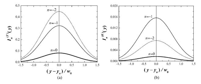
Figure 10. Transverse intensity structure of (a) transmitted  $I_n^{(T)}(y)$  and (b) reflected  $I_n^{(R)}(y)$  beams of various diffraction orders in the planes x = h + L and x = -L, respectively, computed relative to the middle of every beam  $y_n$  at the diffraction of the TE polarized beam with the parameter of tangential propagation  $\beta_0 = 0.64275$  by a rectangular relief grating without a substrate.
