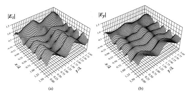
Figure 3. Spatial distribution pattern for the electric field amplitudes  $E_z$  and  $E_y$  of the TE and TM polarizations, respectively, in a planar sinusoidal grating without a substrate in the case of a plane diffracting wave.
