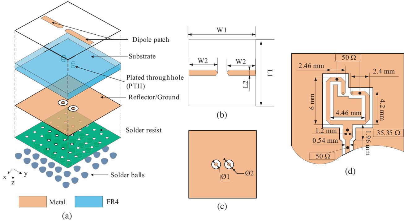
**Figure 1.** Geometry of the proposed antenna element. (a) Exploded view. (b) Top view. (c) Bottom view. (d) Evaluation board.
