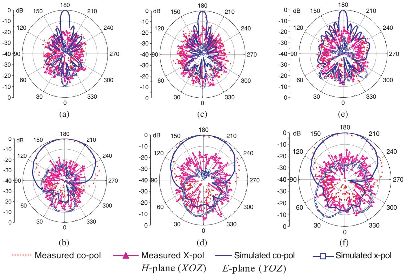
**Figure 6.** Measured and simulated normalization radiation patterns of the antenna element and array. (a)  $f = 26$  GHz, *E*-plane. (b)  $f = 26$  GHz, *H*-plane. (c)  $f = 28$  GHz, *E*-plane. (d)  $f = 28$  GHz, *H*-plane. (e)  $f = 30$  GHz, *E*-plane. (f)  $f = 30$  GHz, *H*-plane.
