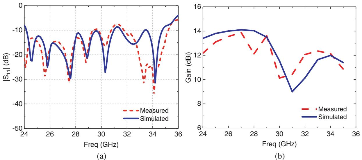
**Figure 5.** (a) Measured and simulated  $|S_{11}|$  of the prototype. (b) Measured and simulated gain of the prototype.
