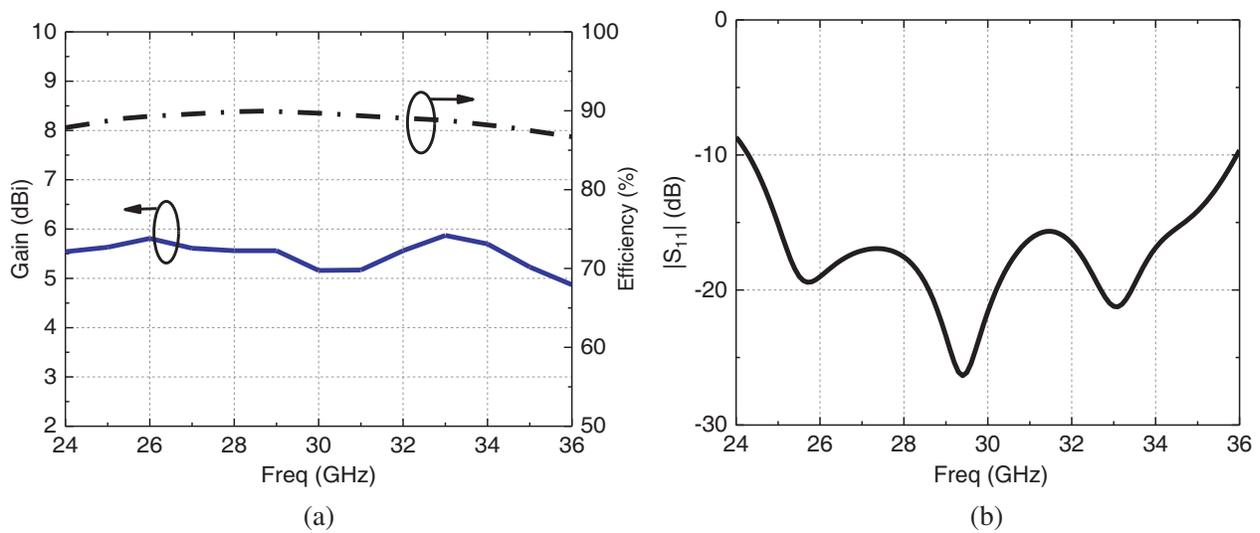
Figure 3. (a) Simulated gain and efficiency of the proposed element. (b) Simulated reflection coefficient of the proposed element.
