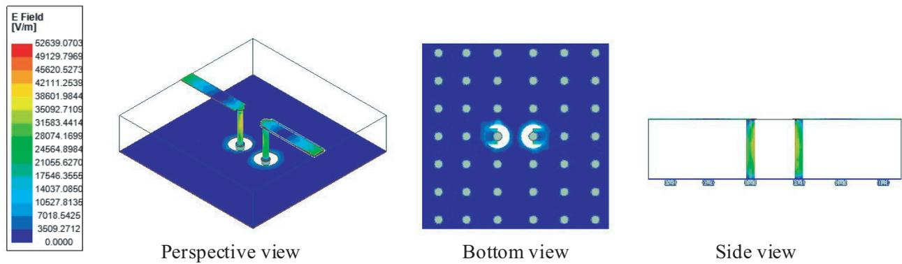
Figure 2. E-field distribution of the antenna element at 28 GHz.
