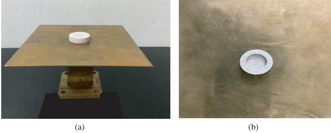
Figure 6. (a) Side view of prototype. (b) Inner side of hollow CDRA.
