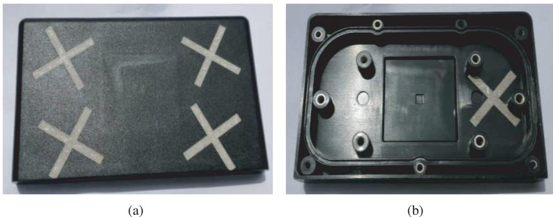
**Figure 7.** Photo of the radome with “X” parasitic structures. (a) Top view. (b) Bottom view.
