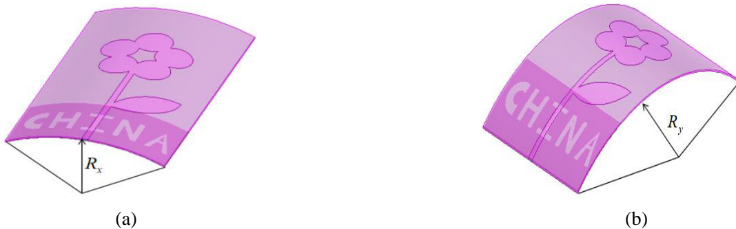
Figure 12. Bionic pear flower shaped antenna structure after bending. (a) Bend along the X axis; (b) Bend along the Y axis.
