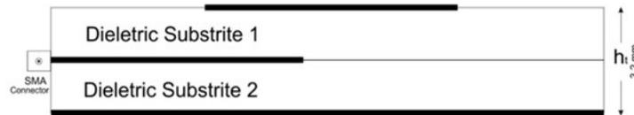
**Figure 5.** Side view of the proposed proximity fed David fractal  $2 \times 1$  patch array antenna with DGS.
