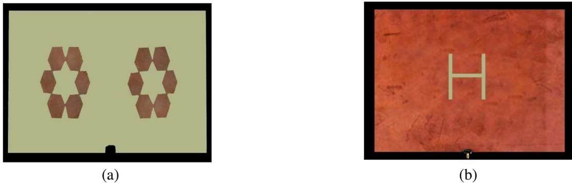
**Figure 6.** Photograph of the fabricated proximity fed David fractal  $2 \times 1$  patch array antenna with DGS, (a) top view and (b) bottom view.
