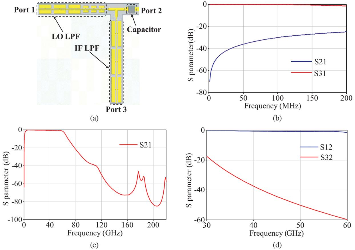
**Figure 4.** Model of the diplexer and simulation results of transmission performance. (a) Model of diplexer circuit. (b)  $S_{21}$  and  $S_{31}$  with the frequency below 200 MHz. (c)  $S_{21}$  with the frequency below 220 GHz. (d)  $S_{12}$  and  $S_{32}$  with the frequency of 30–60 GHz.
