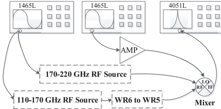
**Figure 9.** Measurement system of the mixer.
