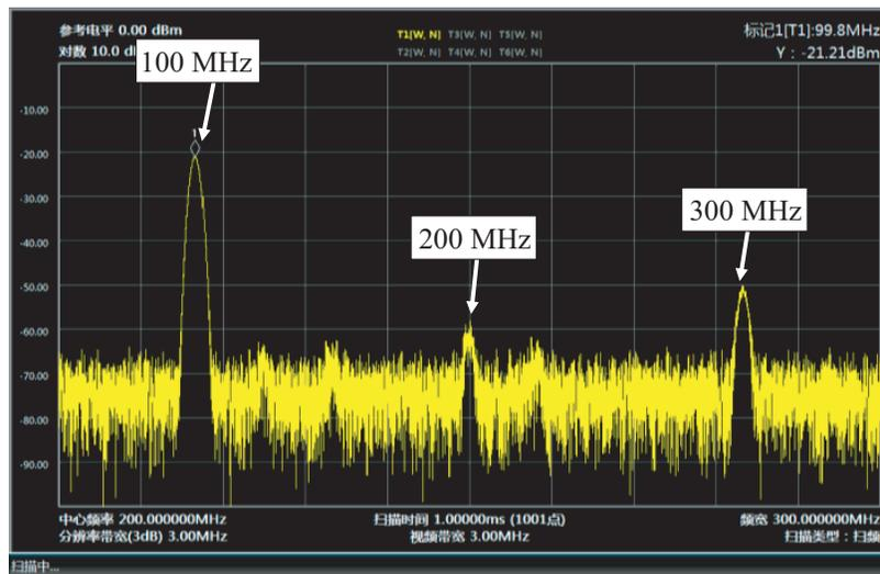
Figure 10. Measured harmonic contents of the mixer.
