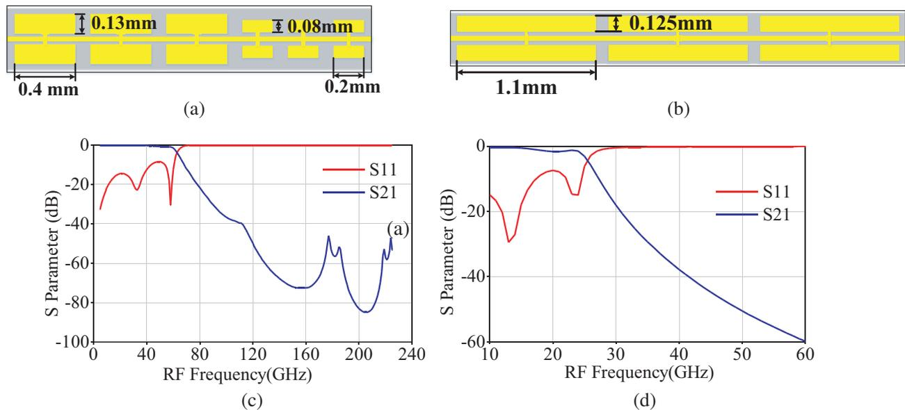
**Figure 3.** Structure of LPFs and simulation results of transmission performance. (a) Structure of LO LPF. (b) Structure of IF LPF. (c) Transmission performance of LO LPF. (d) Transmission performance of IF LPF.
