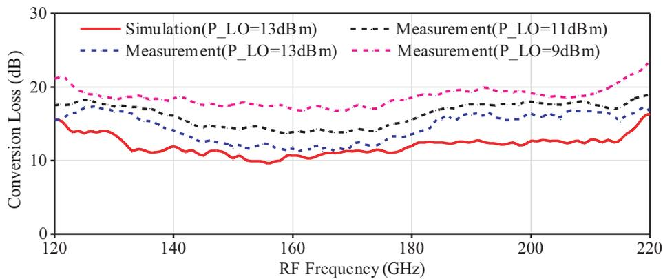
Figure 11. Simulated and measured conversion loss of the mixer.
