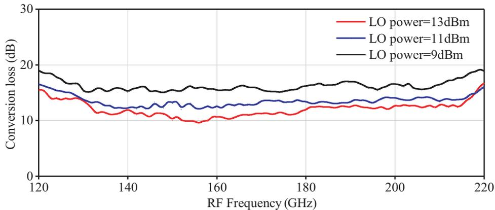
**Figure 5.** Simulation conversion loss with different LO power.
