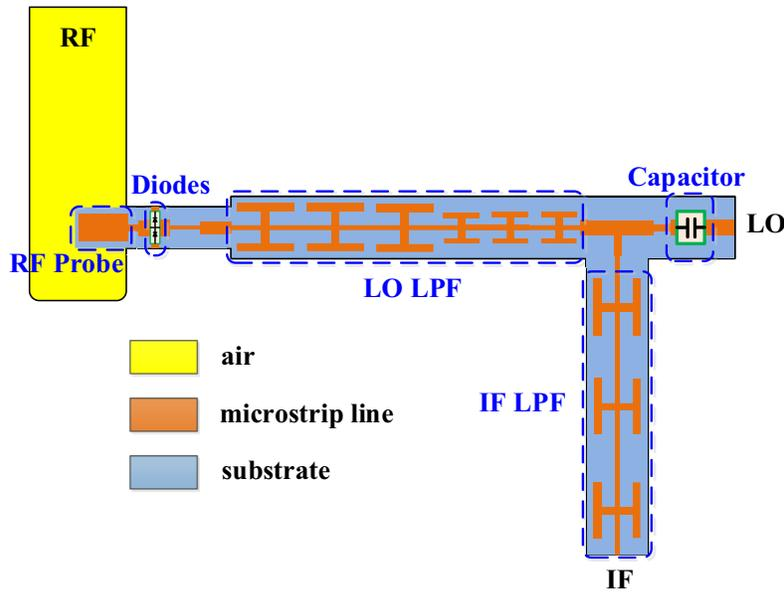
**Figure 2.** Configuration of the proposed mixer.
