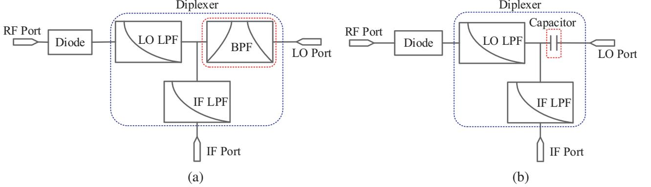
**Figure 1.** Topology diagrams of mixer. (a) Topology of traditional mixer. (b) Topology of proposed mixer.
