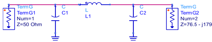
Figure 9. The Pi matching network between 50\ \Omega and 76.5 - j179\ \Omega port impedance terminations for S -parameters.
