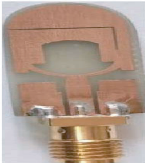
Figure 10. Fabricated prototype of the proposed antenna.
