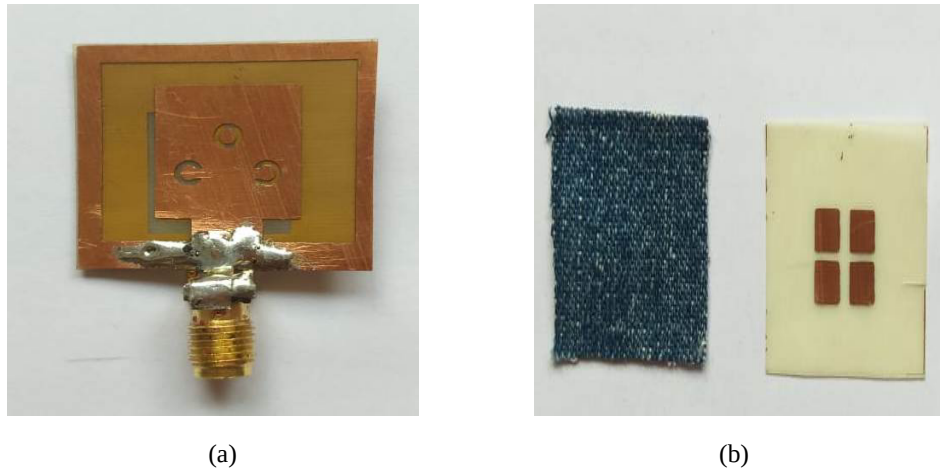
Figure 17. Step 4: Textile gap coupled antenna. (a) Fabricated Antenna-4 Bottom view. (b) Fabricated Antenna-4 EBG and Jeans Used.
