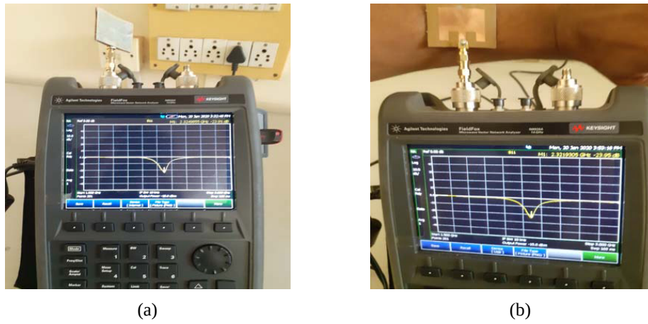
Figure 14. Textile gap coupled antenna. (a) Measured Return Loss. (b) Measured Return loss in vicinity of human hand.
