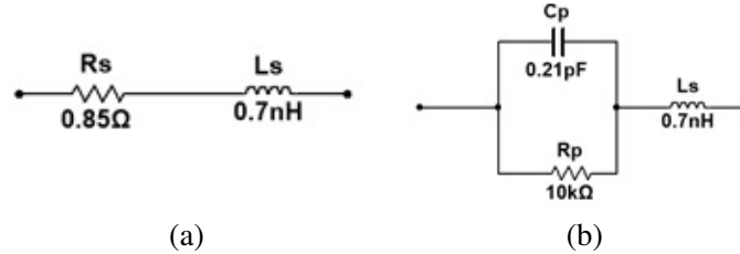
Figure 10. Equivalent circuit of PIN diodes, (a) ON state and (b) OFF state.
