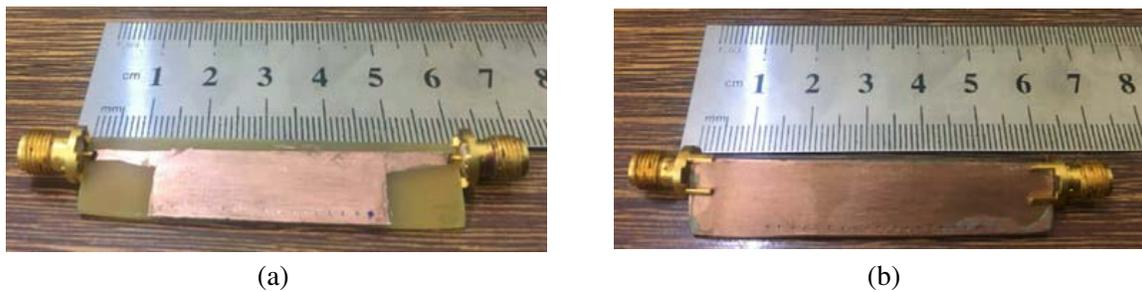
**Figure 5.** The photograph of the fabricated HMSIW high pass filter.
