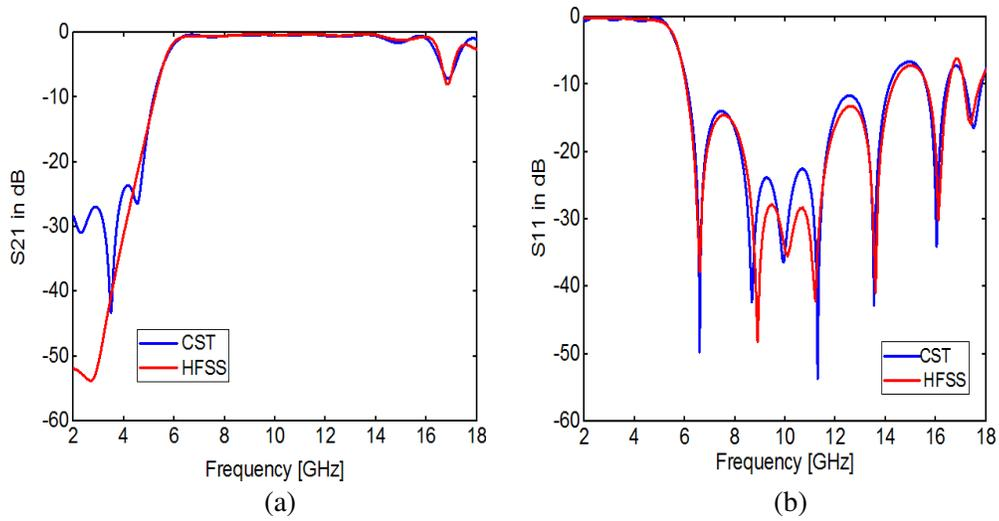
**Figure 3.** (a) Transmission coefficient and return loss of HMSIW filter. (b) Transmission coefficient and return loss of HMSIW filter.
