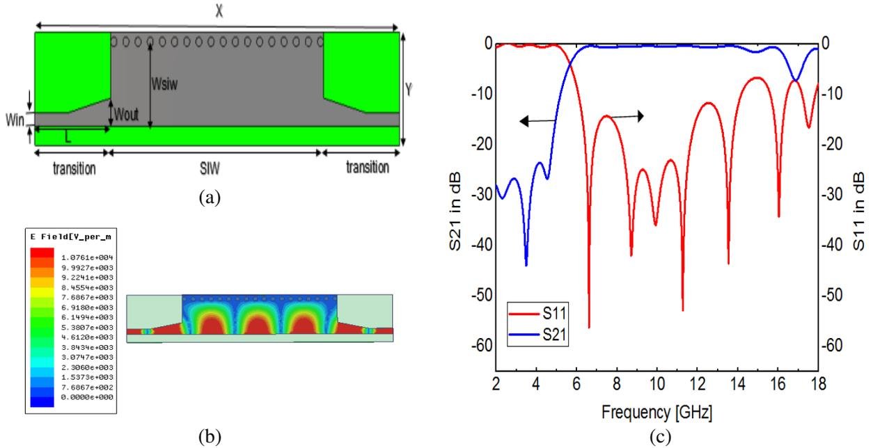
**Figure 2.** (a) Structure of HMSIW high pass filter. (b) Distribution of the electric field at the frequency of 6.1 GHz. (c) Transmission coefficient and return loss of HMSIW filter. The optimized parameters of the HMSIW high pass filter are set such as:  $W_{in} = 1.5$ ,  $W_{out} = 2.5$ ,  $L = 12.5$ ,  $X = 60$ ,  $Y = 12$ ,  $W_{siw} = 9$ .
