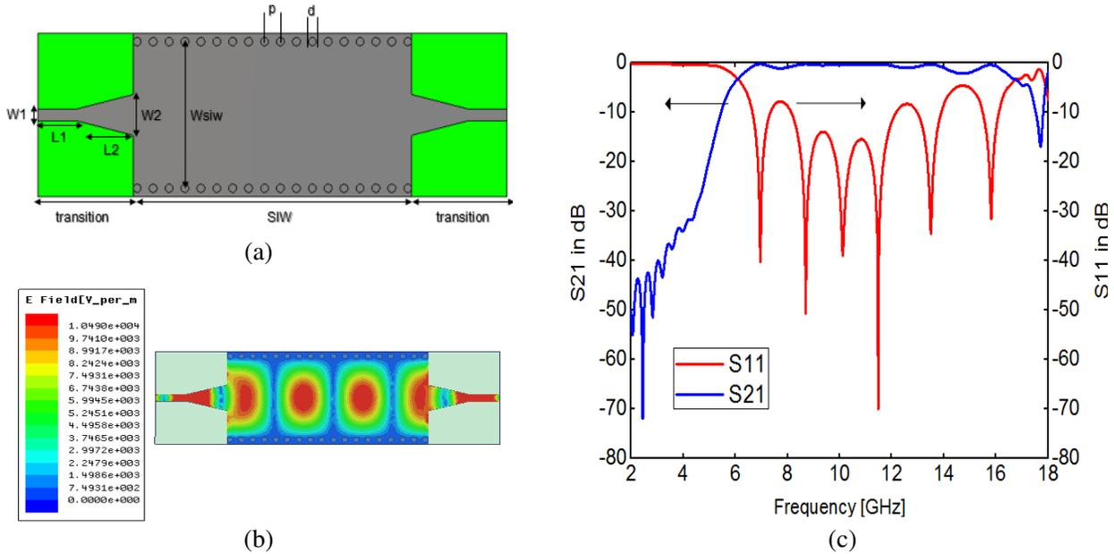
**Figure 1.** (a) Geometry of the SIW high pass filter configuration. (b) Distribution of the electric field at the frequency of 11.5 GHz. (c) Transmission coefficient and return loss of high pass filter. The optimized parameters values of the proposed filter are given in mm such as:  $W_1 = 1.5$ ,  $W_2 = 5.0$ ,  $L_1 = 5.0$ ,  $L_2 = 7.5$ ,  $W_{siw} = 18$ ,  $p = 1.8$ ,  $d = 0.9$ .
