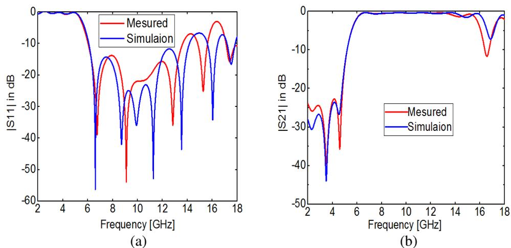
**Figure 6.** (a) Return loss of the HMSIW high pass filter. (b) Transmission coefficient of the HMSIW high pass filter.
