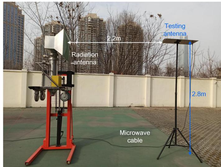
**Figure 1.** Layout of the testing experiment.
