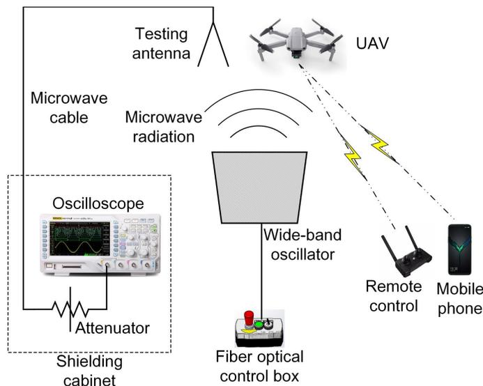
**Figure 4.** Layout of the experiment.
