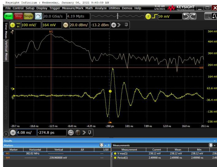
Figure 2. Time-domain waveform and the corresponding FFT waveform of the single pulse.
