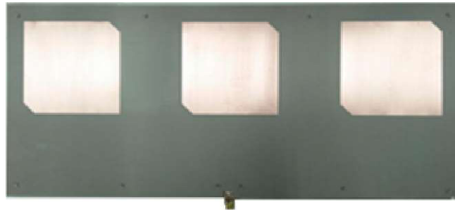
Figure 7. Printed antenna on two layers of Nippon Pillar (NPC-H220A).
