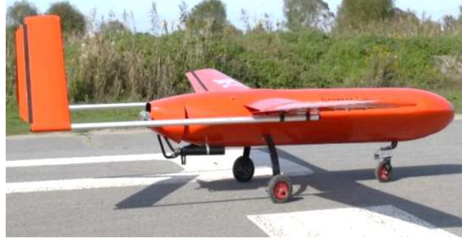
Figure 1. Photograph of our UAV for CP-SAR having total length 4.75 m, wingspan 6 m, and maximum payload 25 kg.
