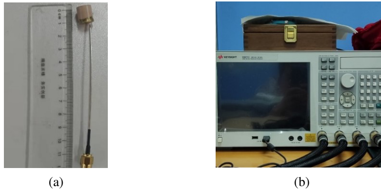
Figure 4. Processing and testing of antenna, (a) antenna object, (b) Agilent e5071c RF network analyzer, (c) simulation and test of antenna S_{11} .
