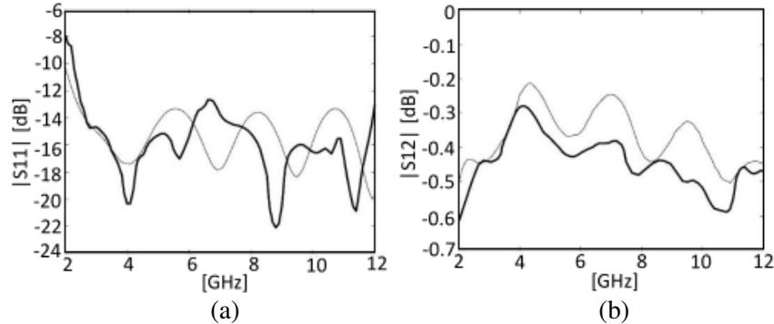
**Figure 8.** Scattering parameters  $|S_{11}|$  and  $|S_{21}|$  of the current project extracted from measurements data (thick line) compared to extracted from numerical model (thin line).
