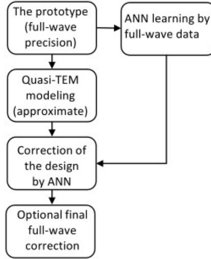
**Figure 1.** The flowchart of the design procedure.
