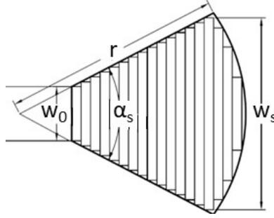
**Figure 2.** Layout of microstrip stub.
