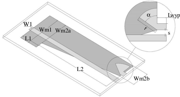
**Figure 4.** UWB microstrip balun structure.
