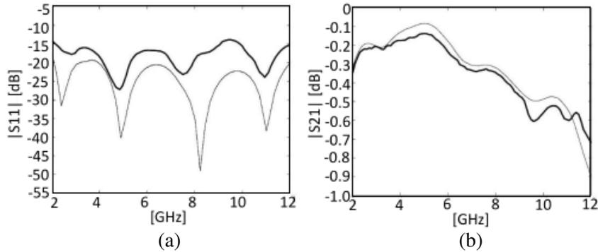
**Figure 7.** Scattering parameters  $S_{11}$  and  $S_{21}$  of the prototype extracted from measurements data (thick line) compared to extracted from numerical model (thin line).
