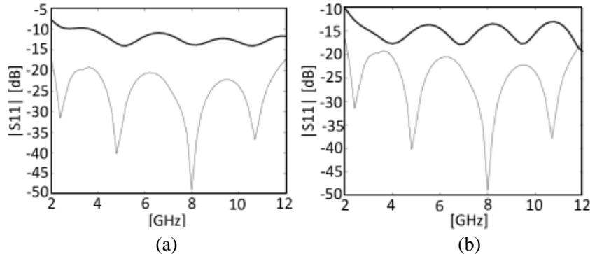
**Figure 5.** Reflection coefficients of the balun designed on RT Duroid 6006 (thick line) compared to the prototype designed on RF-45 (thin line) (a) after application of the scaling procedure; (b) after application the scaling and ANN.
