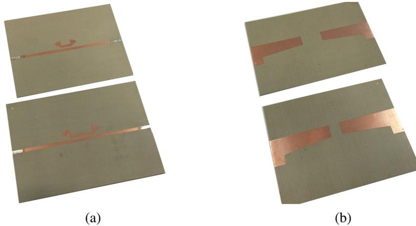
**Figure 6.** The photos of baluns in b2b configurations: straightway and by quarter-wave line according to [14], (a) top view, (b) bottom view.
