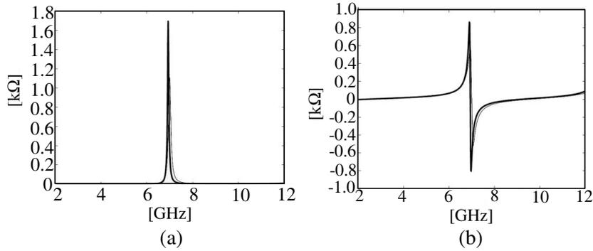
**Figure 3.** The resistances and the reactances of the prototype (thick lines) and the current project (thin lines) for the exemplary microstrip stub, (a) resistance, (b) reactance.
