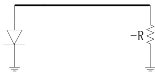
Figure 3. Schematic of a transmission line with nonlinear oscillator.
