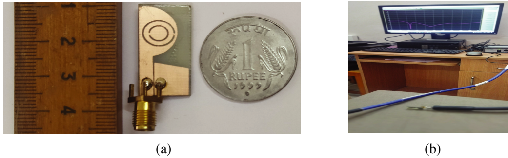
Figure 5. (a) Fabricated antenna. (b) Measurement setup.
