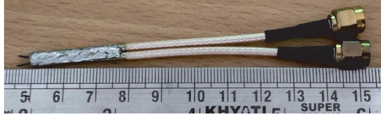
Figure 9. Semi-rigid differential probe used for impedance measurement.
