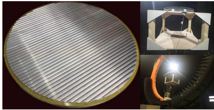
Figure 7. Diagram of the manufacturing antenna and test environment.
