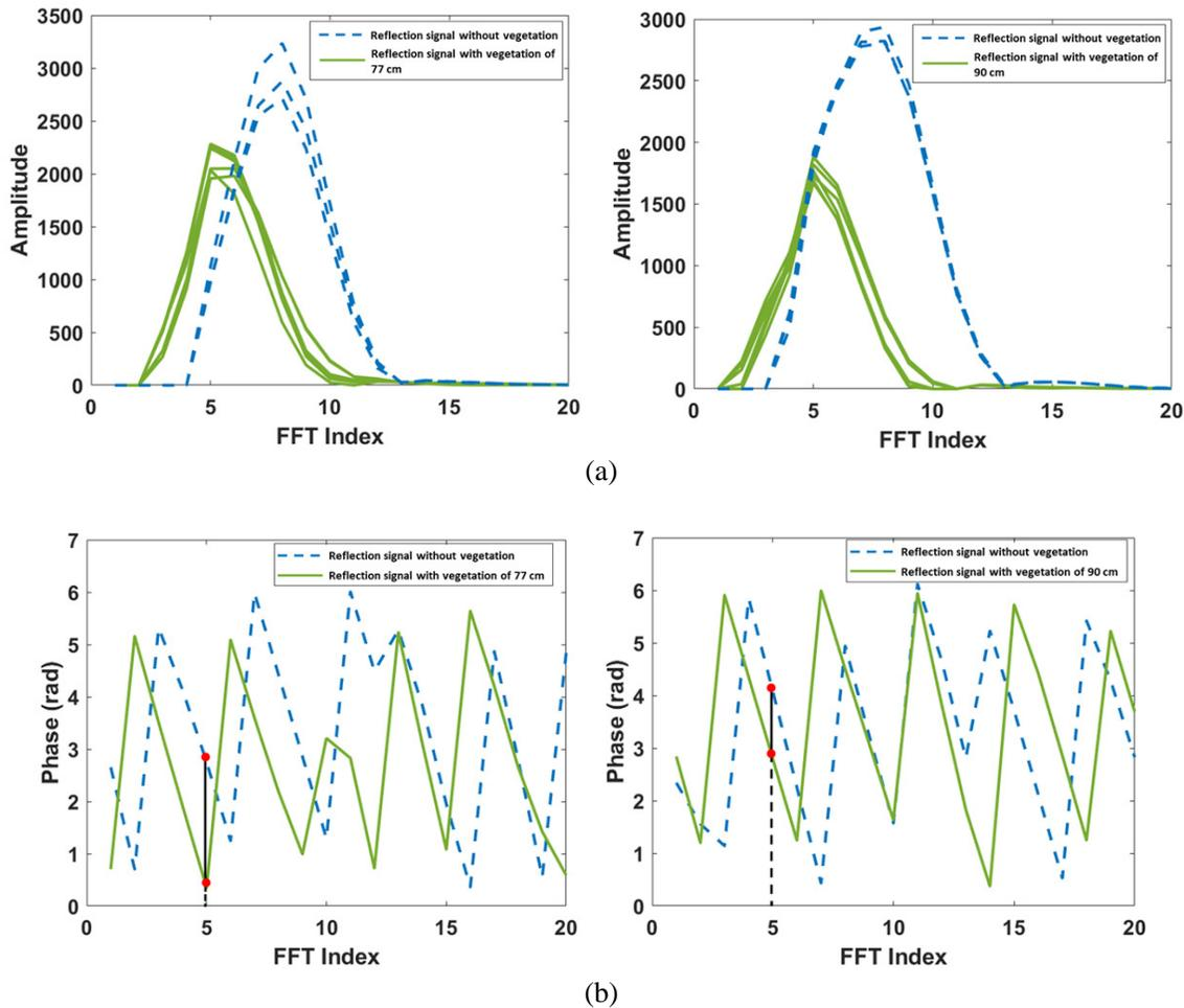
**Figure 9.** Reflected signal received by the radar system with and without vegetation. (a) Magnitude of reflected signal. (b) Phase of reflected signal.
