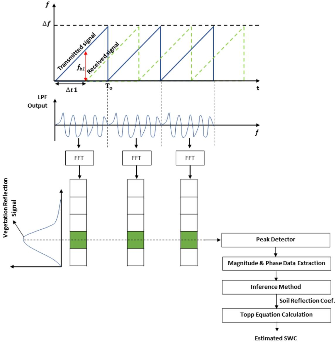
**Figure 3.** The proposed flow of the SWC estimation using FMCW radar.
