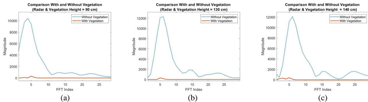
**Figure 10.** Comparison of measurement results with and without vegetation with the same height of radar and vegetation. (a) 90 cm. (b) 130 cm. (c) 140 cm.
