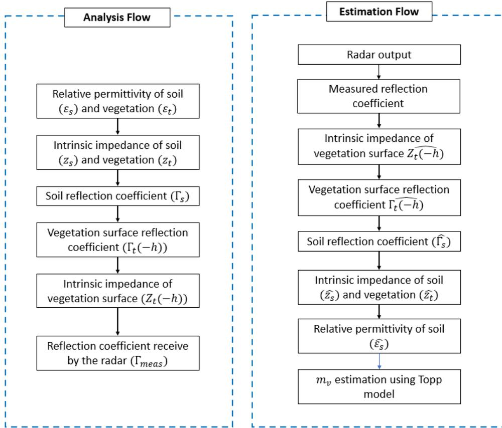
**Figure 6.** Flowchart of estimation of soil relative permittivity.
