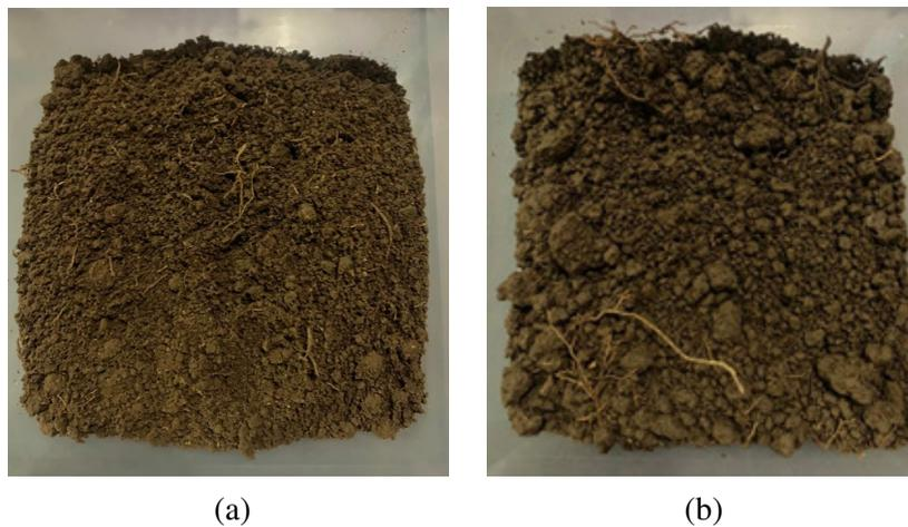
**Figure 13.** Differences in soil texture with different values of soil water content. (a) SWC = 40%. (b) SWC = 47%.
