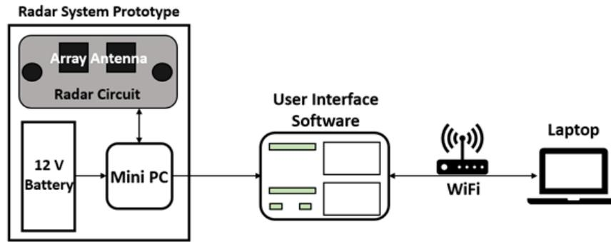
**Figure 7.** Realization of the FMCW radar system for estimating SWC.
