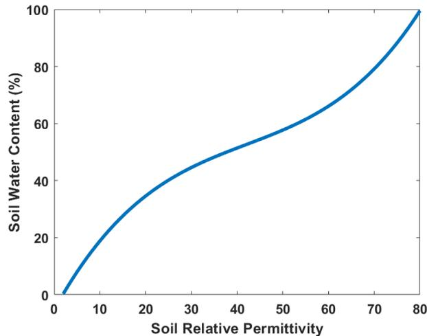
**Figure 4.** The relationship between soil permittivity and SWC based on the Topp equation [30].
