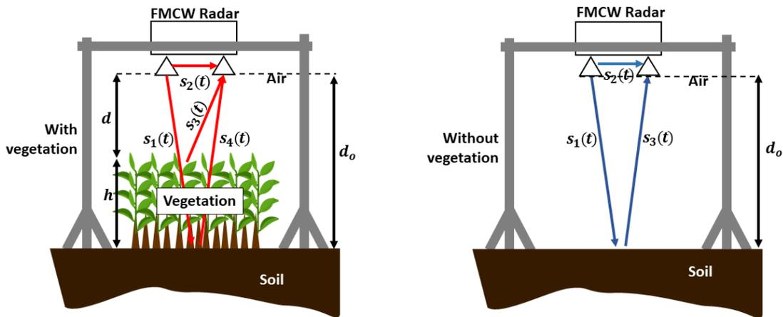
Figure 1. Concept of measuring the SWC using the proposed FMCW radar system.
