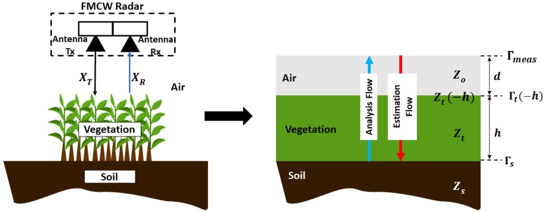
**Figure 5.** Illustration of flow analysis and estimation of soil relative permittivity using a radar system.
