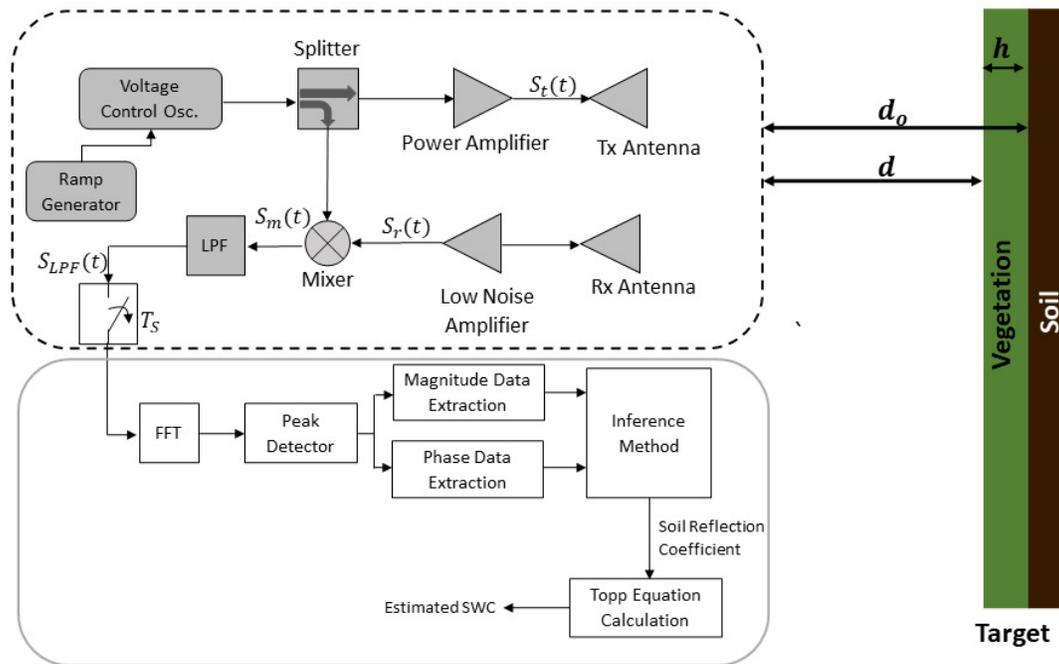
Figure 2. Block diagram of the proposed FMCW radar for SWC estimation.
