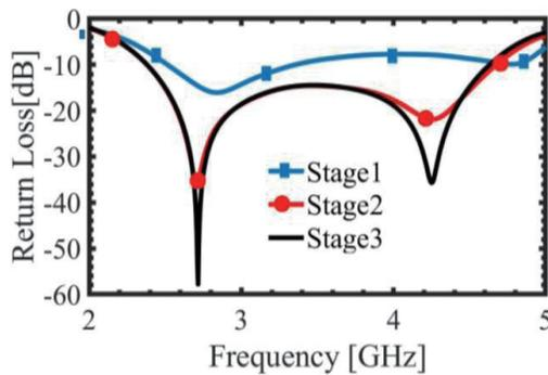
**Figure 3.** Comparison of return loss characteristics in different evolution stages.
