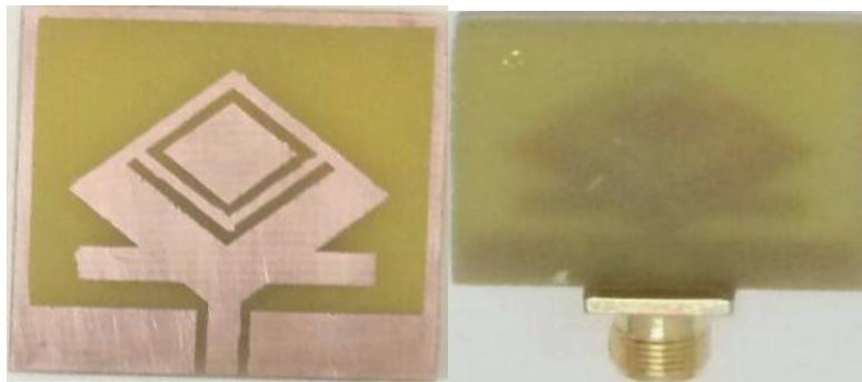
**Figure 8.** Prototype of front & back view of proposed diamond shape antenna.
