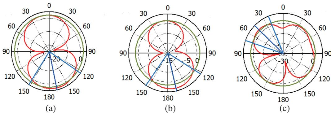
**Figure 13.** Gain Pattern of Proposed Antenna at (a) 2.4 GHz (b) 3.5 GHz. and (c) 4.5 GHz.
