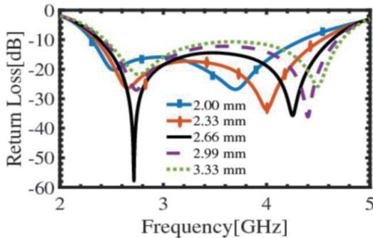
**Figure 5.** Results of variations of width ( $S_{11}$ ) of rectangular slit on the  $S$ -parameters.
