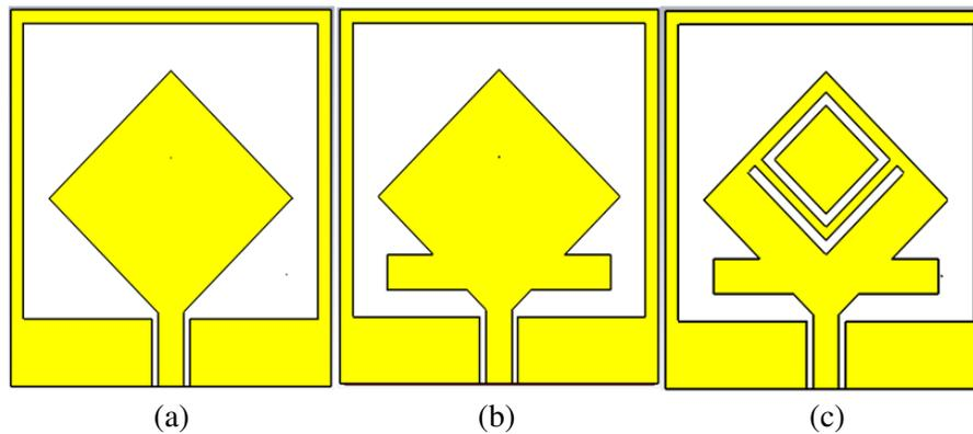
**Figure 2.** Design evolution stages I, II, and III of the proposed diamond shaped antenna. (a) Stage-I. (b) Stage-II. (c) Stage-III.
