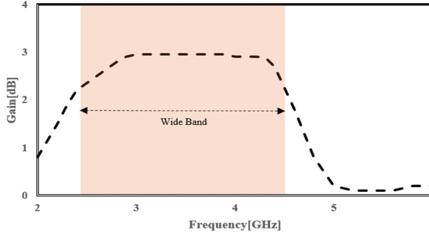
**Figure 11.** Gain versus frequency graph of proposed diamond shape antenna.
