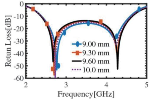
**Figure 6.** Results of variations in the outer ring ( $D$ ) of Diamond shape primary patch.
