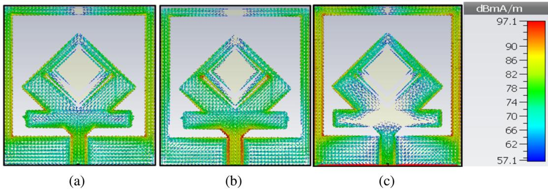
**Figure 12.** Effect of surface current dispersals of the projected antenna at changed frequencies 2.4 GHz, 3.5 GHz, and 4.5 GHz. (a) 2.4 GHz, (b) 3.5 GHz, (c) 4.5 GHz.
