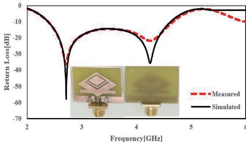
**Figure 9.** Measured and simulated results of the proposed diamond shape antenna.
