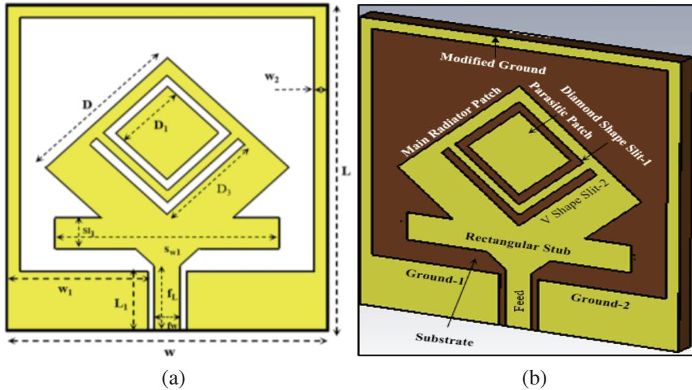
**Figure 1.** Proposed circularly polarized diamond-shaped wideband antenna. (a) 2D and (b) 3D view.
