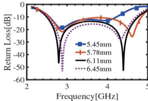
**Figure 7.** Results of variations in position V Shape Slit for the proposed antenna.
