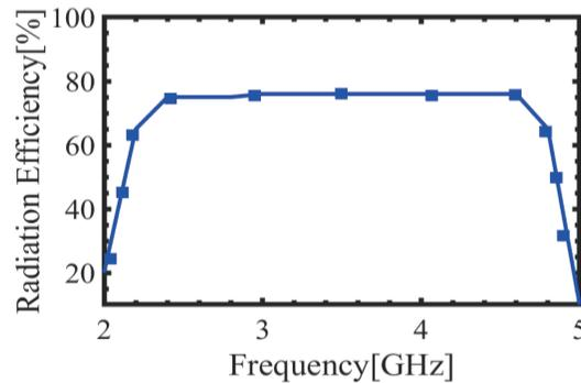
**Figure 14.** Radiation efficiency of proposed diamond shape antenna.
