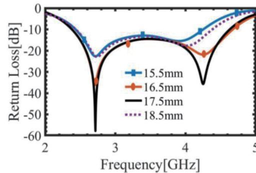
**Figure 4.** Results of variations of width ( $S_{W1}$ ) of rectangular slit on the  $S$ -parameters.
