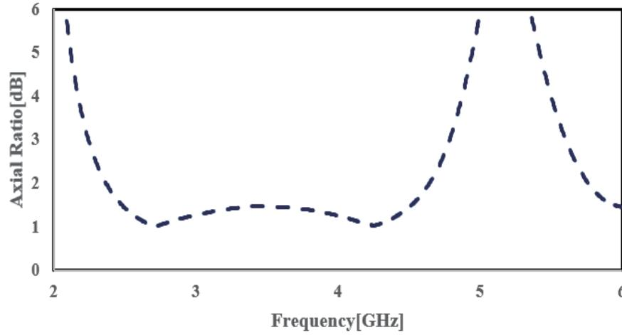
**Figure 10.** Axial ratio of proposed diamond shape antenna.
