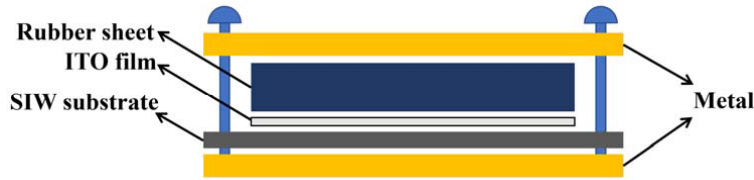
Figure 2. Assembling method of SIW equalizer.
