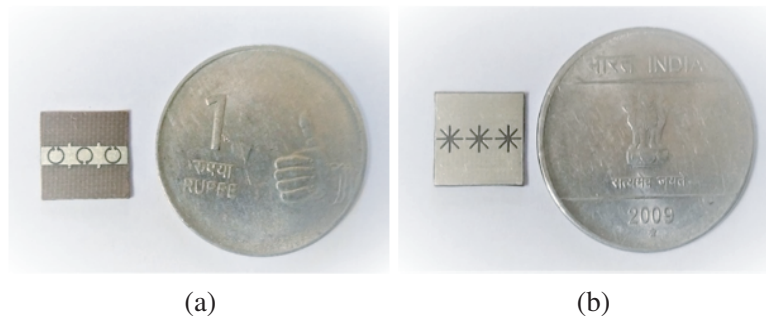
Figure 13. Photograph of fabricated model of presented filter. (a) Top view. (a) Bottom view.
