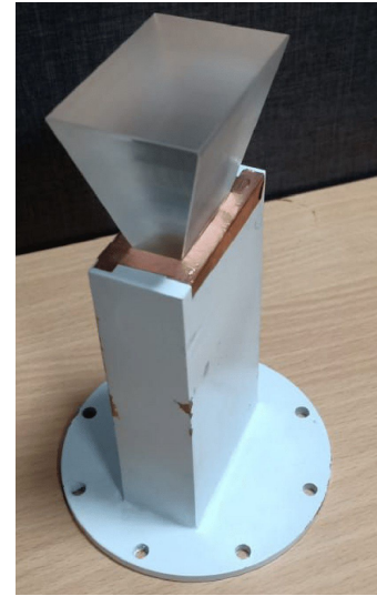
FIGURE 18. Fabricated antenna with tapered transition as in [15].
