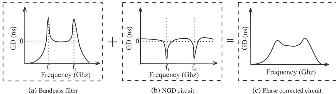
**Figure 1.** GD equalization in bandpass filter using NGDC [1].
