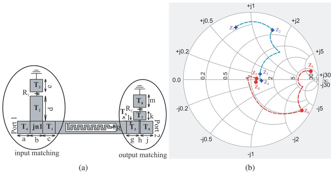
**Figure 3.** Proposed low-loss pulse-shaped stub-loaded NGDC with its (a) Top view where  $a = b = c = e = g = j = m = 3$  mm,  $d = 6$  mm,  $h = l = 0.3$  mm and  $k = 2$  mm, (b) Transition of input/output port impedance.
