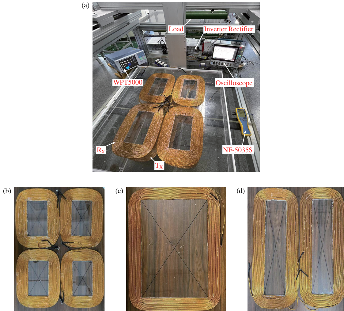
FIGURE 9. Experimental setup. (a) Experimental system diagram. (b) FBISC coil configuration. (c) Conventional coil configuration. (d) DD coil configuration.
