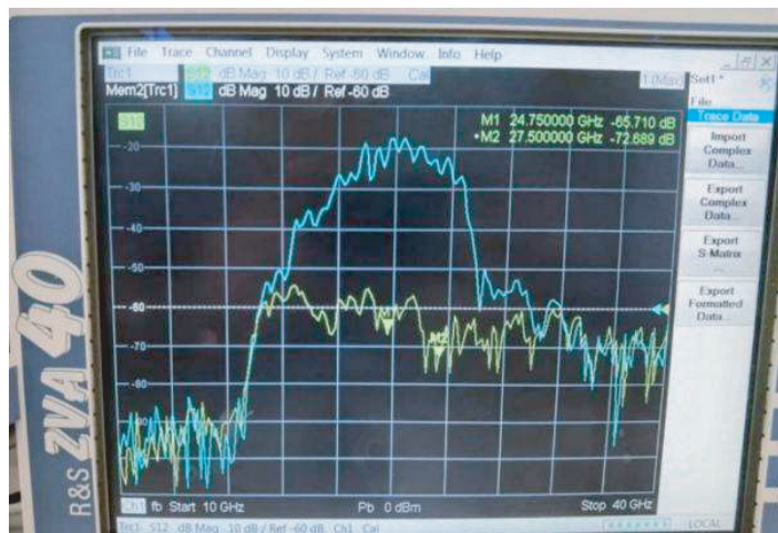
FIGURE 12. Frequency band testing of the active antenna.
