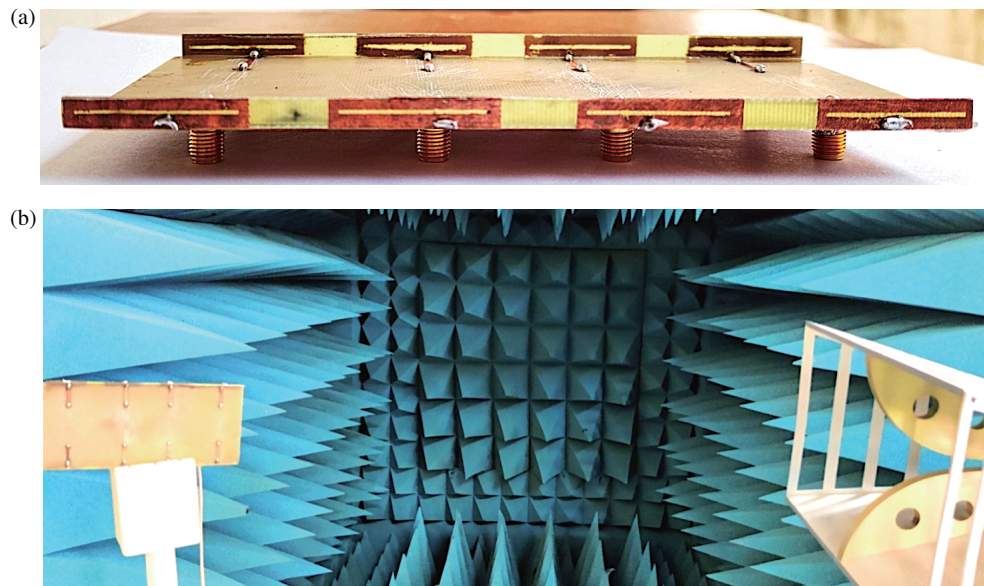
FIGURE 5. Images of (a) developed 8x8 MIMO antenna. (b) Setups for measuring radiation characteristics and efficiency.
