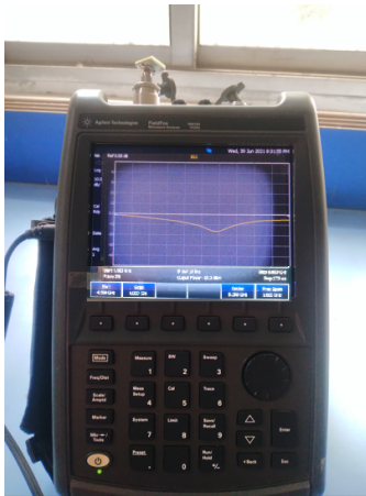
FIGURE 14. Proposed antenna measurement using VNA.
