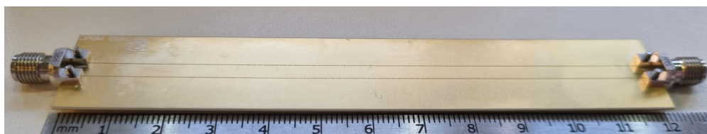
FIGURE 17. SIW with CPWG transition PCB and connectors manufactured.
