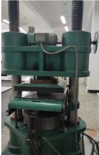
FIGURE A1. Material parameters tension and compression test platform (FL4000).
