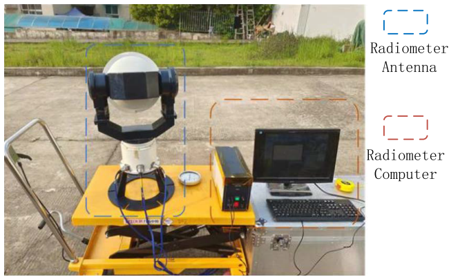
FIGURE 8. 3 mm passive millimetre wave imaging system.
