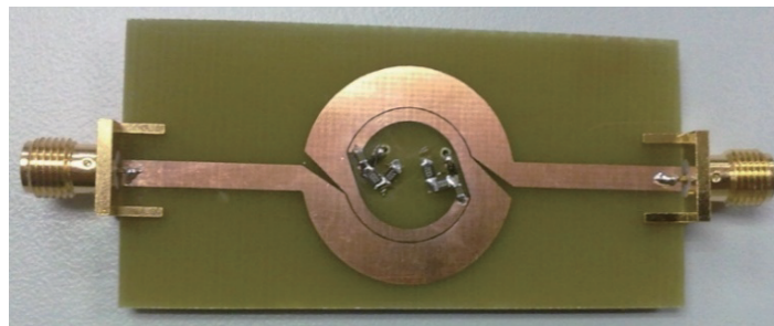
FIGURE 10. Photograph of the fabricated filter on a FR4 substrate.
