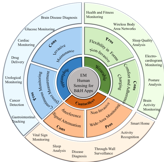
FIGURE 2. Categories of EM-based human sensing technologies, showcasing contactless, wearable, and implantable approaches, their advantages, limitations, and diverse applications in B&H domain.
