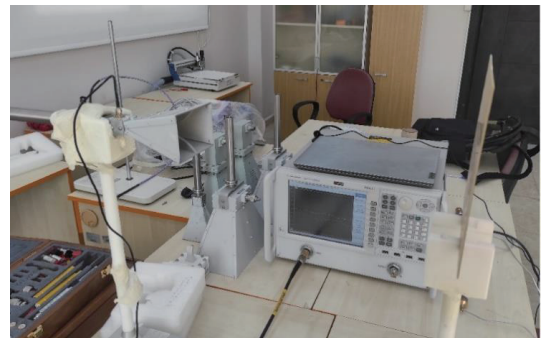
FIGURE 9. Experimental setup for the measurement of absorption.
