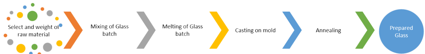
FIGURE 1. Glass manufacture by melt-quenching technique procedure.
