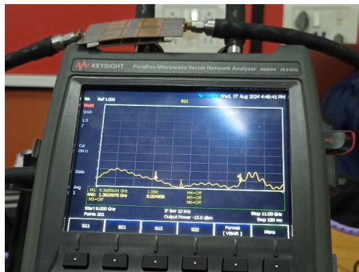
FIGURE 14. Experimental setup for MIMO antenna with AMC patches.
