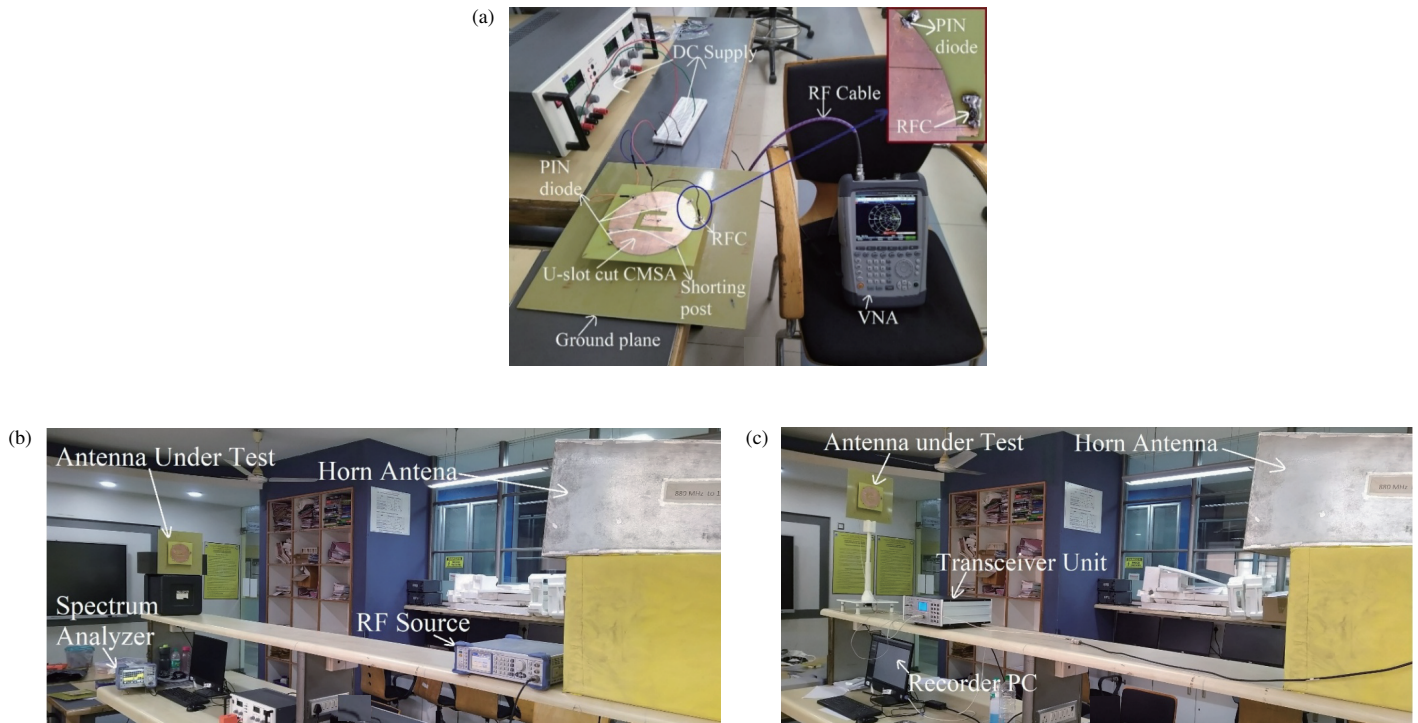
FIGURE 6. (a) S_{11} BW measurement setup, and (b) broadside gain, and (c) radiation pattern measurement setup for reconfigurable design of U-slot cut CMSA.
