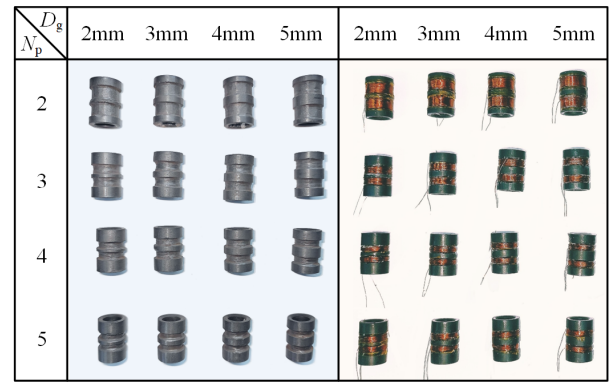
FIGURE 2. The magnetic cores and RCs with different groove spacing ( D_g ) and winding layers ( N_p ).
