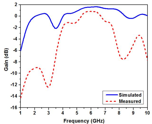
**FIGURE 8.** Gain of the CP monopole antenna.
