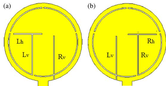
**FIGURE 4.** (a) LHCP configuration. (b) RHCP configuration.
