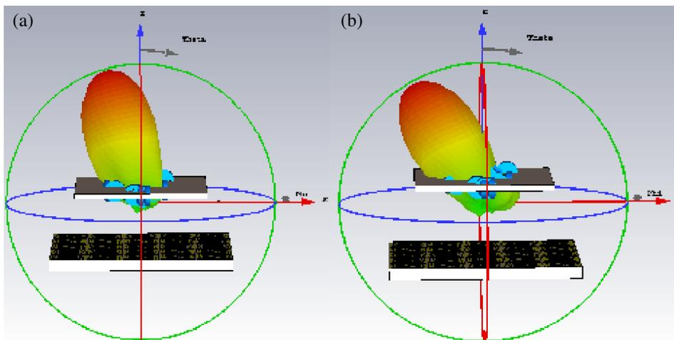
FIGURE 27. 3D view of simulated beam steering. (a) With ZPM (RHCP at -12°). (b) With PGM (RHCP at -27°).
