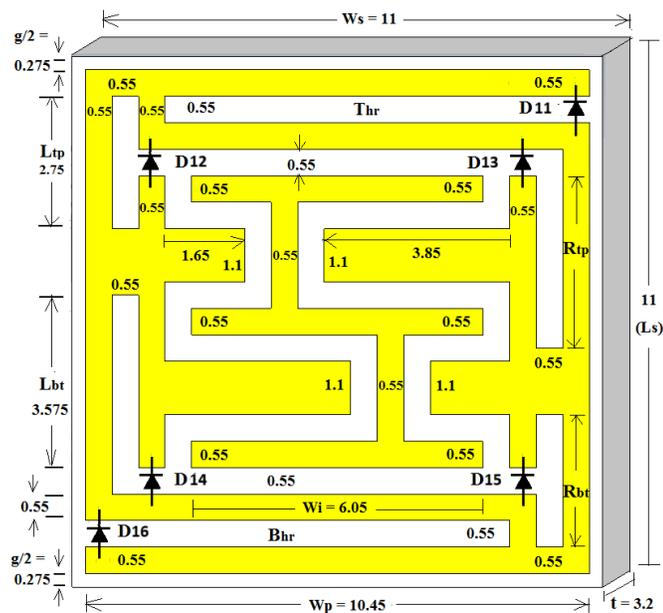
FIGURE 12. Proposed reconfigurable unit cell (Dimensions are in mm).
