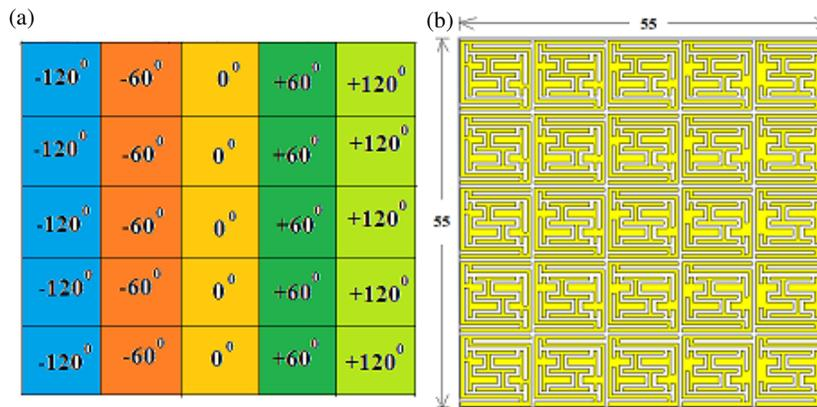
FIGURE 20. PGM at 6 GHz. (a) Diagrammatic representation. (b) Metasurface.
