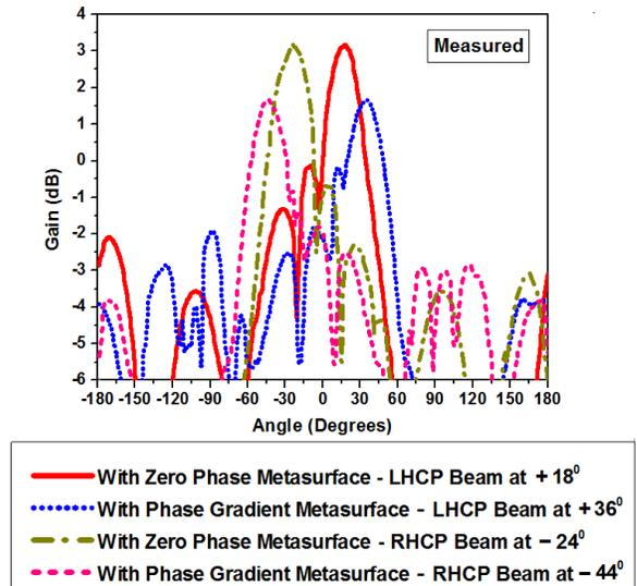
FIGURE 25. Measured beam steering for RHCP and LHCP at 6GHz (2D plot).
