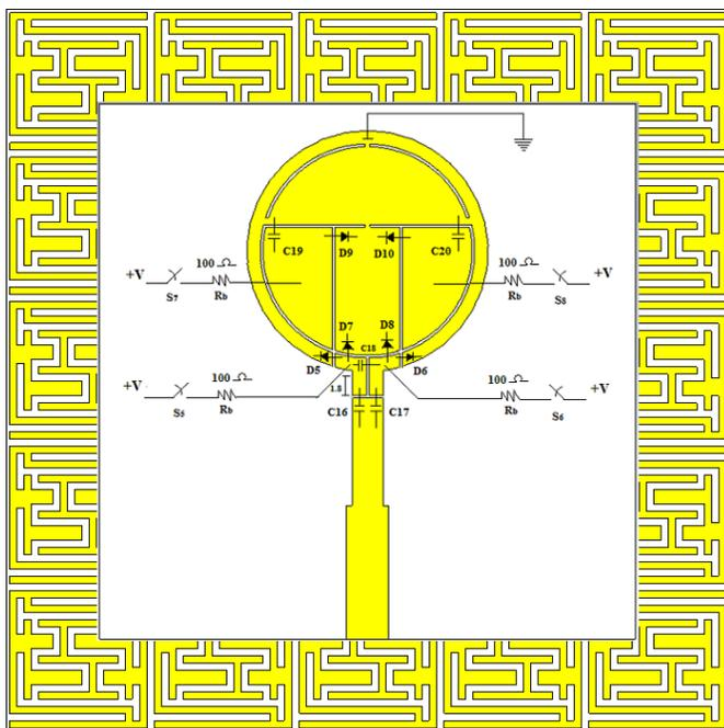
FIGURE 16. Antenna backed by ZPM — Front view.
