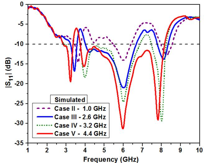
FIGURE 6. Simulated result of  $|S_{11}|$  — NB responses of Case — II, III, IV, and V.
