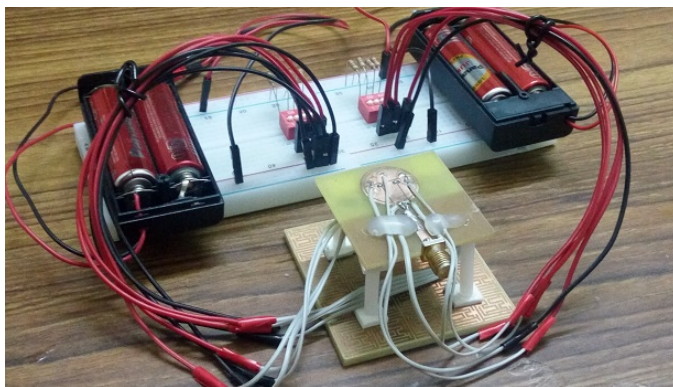
FIGURE 32. Fabricated antenna backed by metasurface, along with a biasing circuit.
