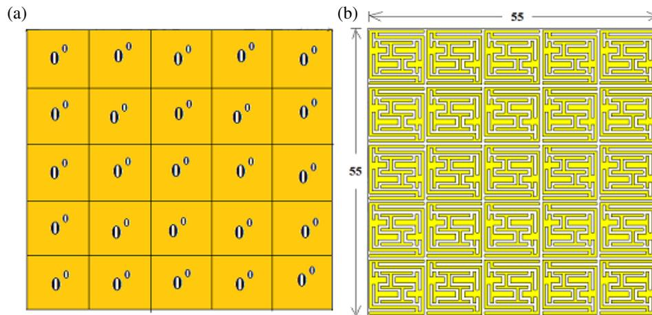
FIGURE 14. ZPM at 6 GHz. (a) Diagrammatic representation. (b) Metasurface.
