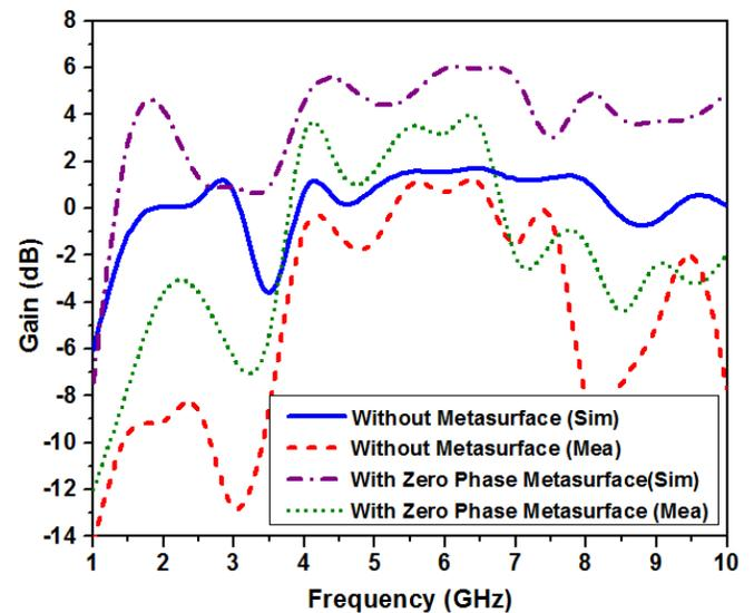
FIGURE 17. Antenna gain, with/without metasurface.
