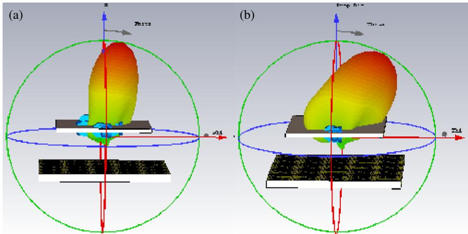
FIGURE 26. 3D view of simulated beam steering. (a) With ZPM (LHCP at +10°). (b) With PGM (LHCP at +23°).
